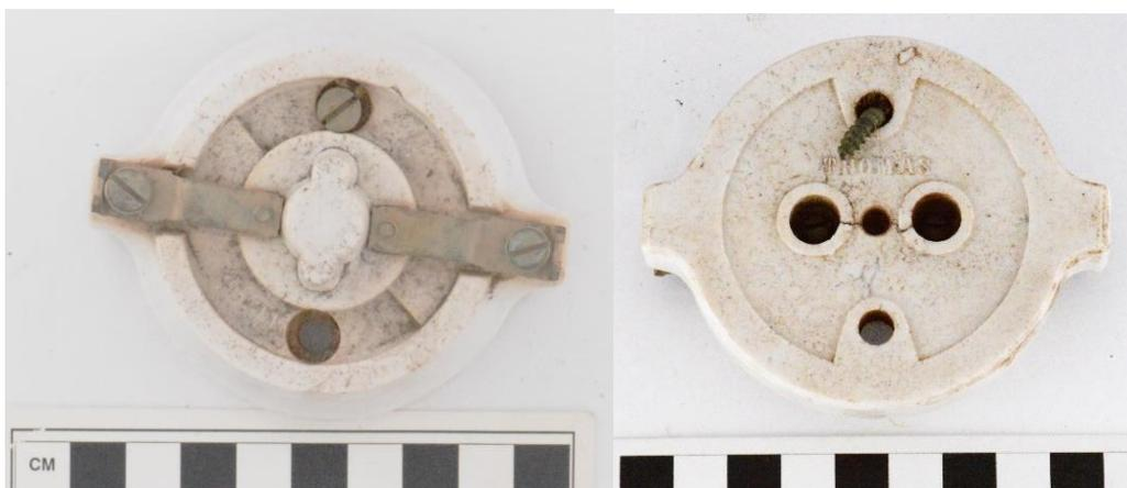
Figure 65. Ceramic fuse holder (23-0017-041).
