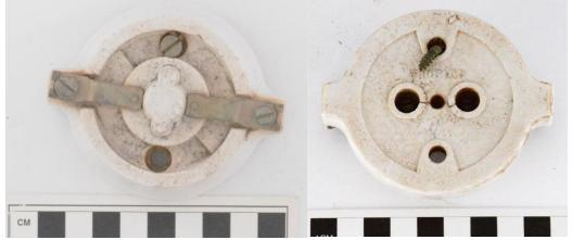
Figure 65. Ceramic fuse holder (23-0017-041).
